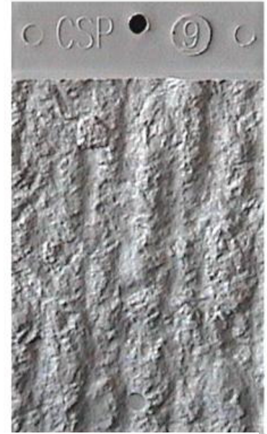
CSP 9 Heavy Scarification
