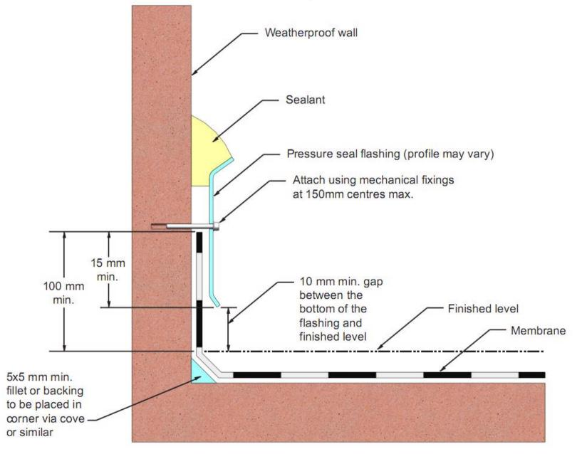
Vertical upward termination – overflashing profile
